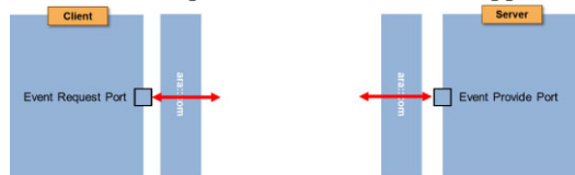
Figure 5 Handling of Events in AUTOSAR Adaptive Application
