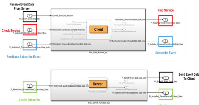
Figure 3 Modelling of event data exchange for AUTOSAR Classic client/server SWCs in Simulink
