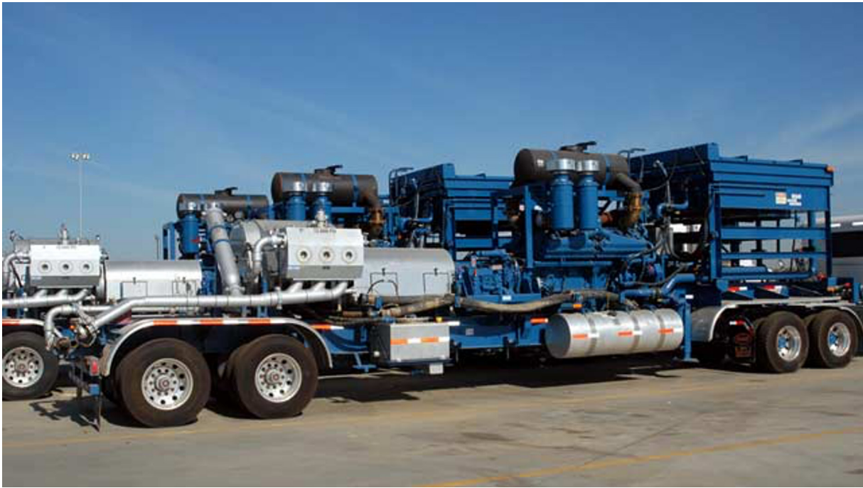
A frac truck which carrying triplex pumps.
